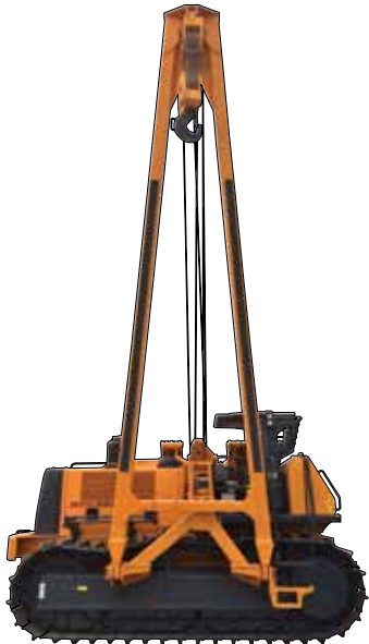
SPX-960 / 960 SV Lifting capacity: 96-ton
