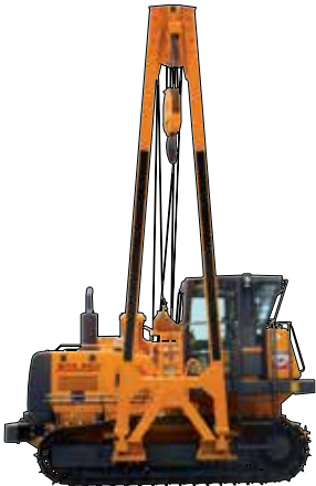
SPX-460 Lifting capacity: 46-ton
