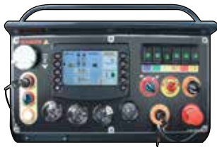
Fig. 3: Control panel: from here the operator monitors speed, travel, pitch, load and other critical information
