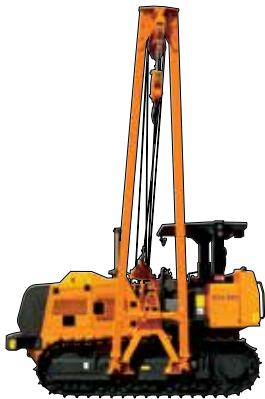
SPX-260 Lifting capacity: 26-ton
