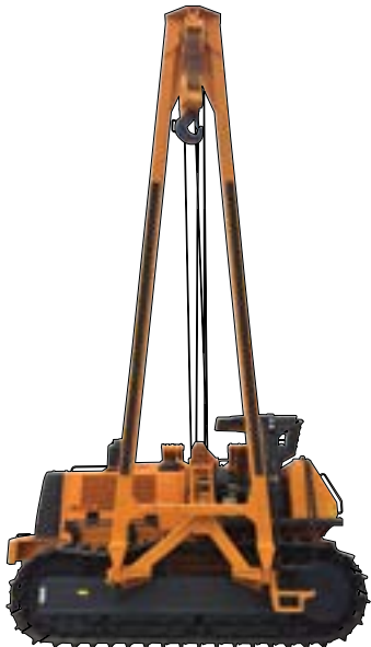
SPX-960 Lifting capacity: 96-ton
