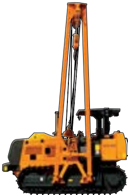
SPX-260 Lifting capacity: 26-ton
