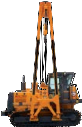
SPX-460 Lifting capacity: 46-ton
