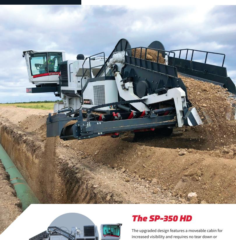
The upgraded design features a moveable cabin for increased visibility and requires no tear down or setup, meaning the machine is ready to work when it arrives onsite. Other enhancements include 4 cameras on the machine to monitor the off-sides, shaker and loading of material, and an upgraded undercarriage for more stability.
