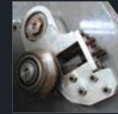
TOOLING The bearing wheel features a number of tool-holding heads. Rotation and forward motion allow these heads to bevel the pipe.
