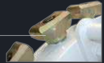
PISTONS Small pistons push into the internal wall of the pipe during clamp opening to allow for the pipe facing machine's alignment.
