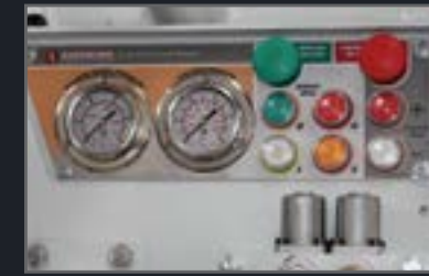
CONTROL PANEL (NOT SHOWN) A control panel allows the operator to control the machine's main functions. An emergency button will block all hydraulic operations without affecting the diesel engine of the power unit.
